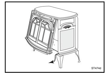
Fig. 65 Remove the Stove Front.
